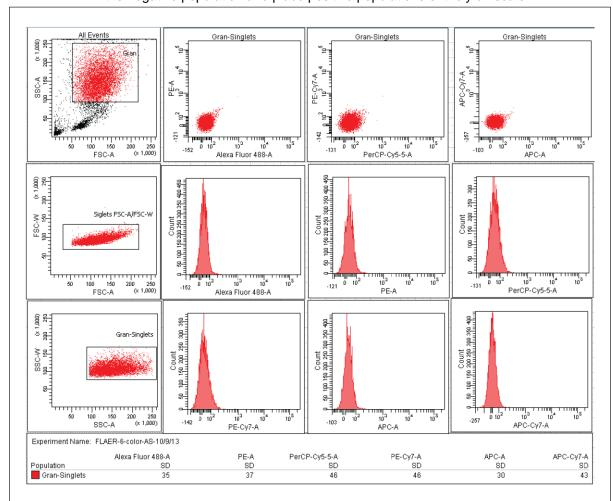
Example of optimal PMT setting for granulocytes ( $\geq$ 2.5 robust standard deviations of the baseline setting) on a BD<sup>TM</sup> FACSCanto instrument.
